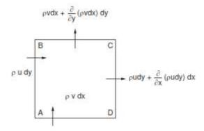
First considering the y-z face, perpendicular to the x direction and located at x, the flow through face during time dt is given by
