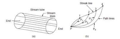
Particles P<sub>1</sub>, P<sub>2</sub>, P<sub>3</sub>, P<sub>4</sub>, starting from point P at successive times pass along path lines shown. At the instant of time considered the positions of the particles are at 1, 2, 3 and 4. A line joining these points is the streak line.
