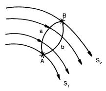
Thus  $\psi_B - \psi_A =$  flow rate between  $S_1$  and  $S_2$ . The flow left to right is taken as positive, in the sign convention. The velocities u and v in x and y directions are given by
